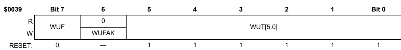
Figure 62. PWU Control/Status Register 0 (PWUCS0)
